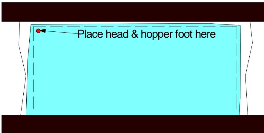
Move Statler head to the upperleft corner of the fabric such that when the pattern sews out the top and left edge will be on the fabric.
