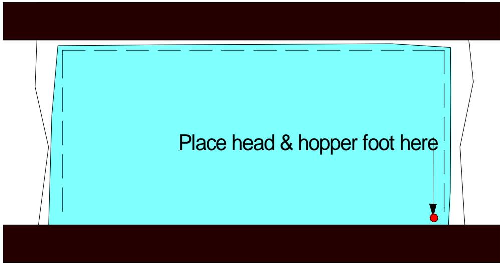
Move the head and hopper foot to the lower right corner of the fabric.
